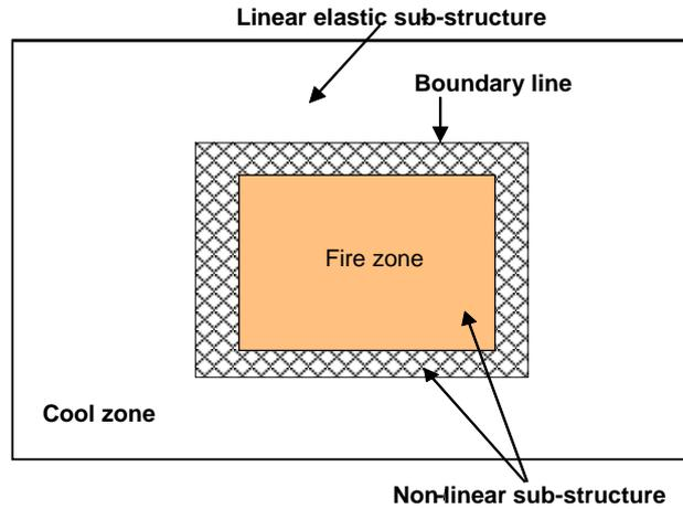
Figure 1: Sub-structuring scheme for structural analysis in fire.
