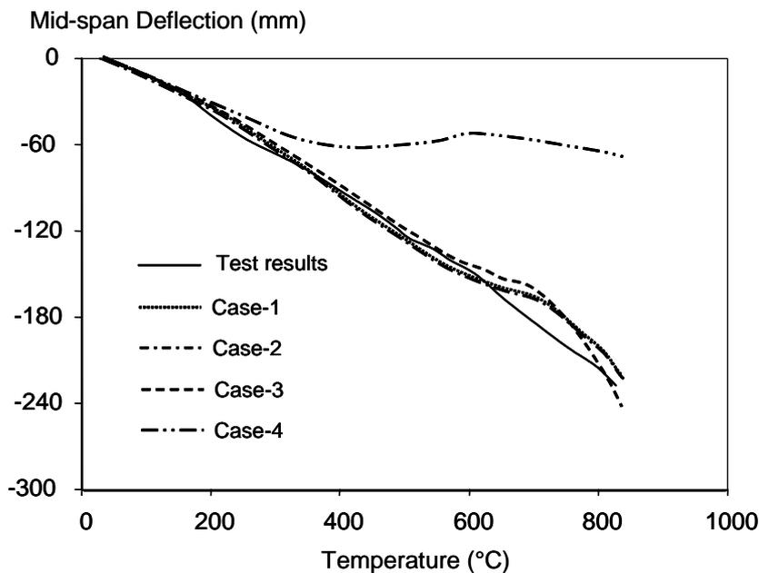
Figure 3 Comparison of predictions with measured mid-span deflections for the different non-linear sub-structures analysed in the Restrained Beam Test
