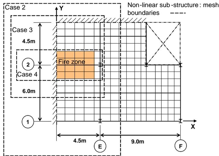
Figure 2 Finite element layout adopted in the analysis for the Restrained Beam Test, together with the boundaries of the non-linear sub-structures for the three cases studied.
