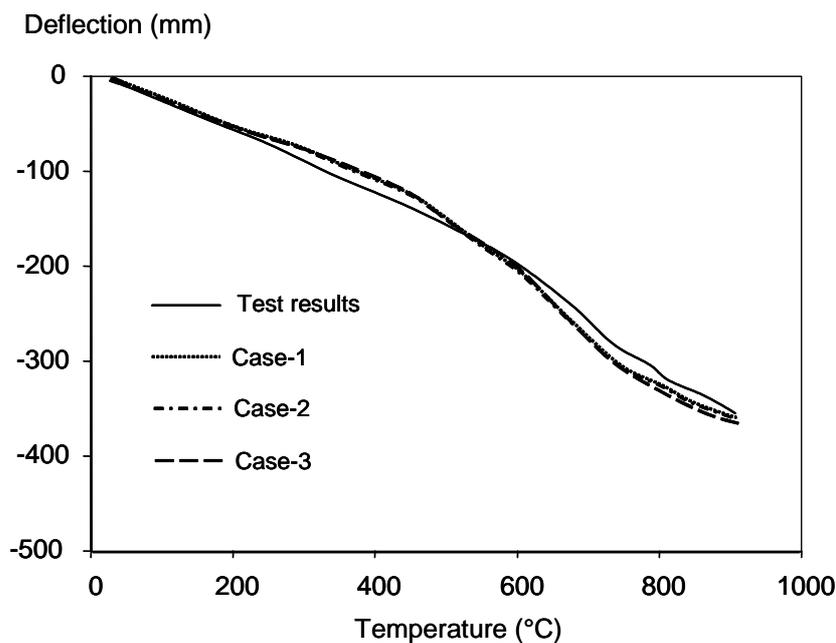
Figure 5 Comparison of predictions with measured deflections at position D11 for different non-linear sub-structures analysed for the British Steel Corner Test
