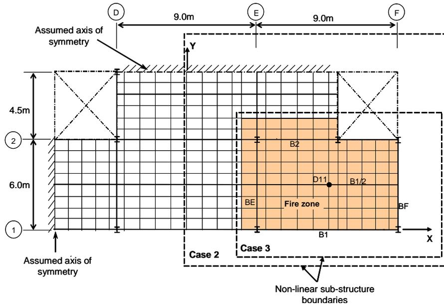
Figure 4 Finite element layout adopted in the analysis for British Steel Corner Test, together with the locations of non-linear sub-structures for the two cases studied
