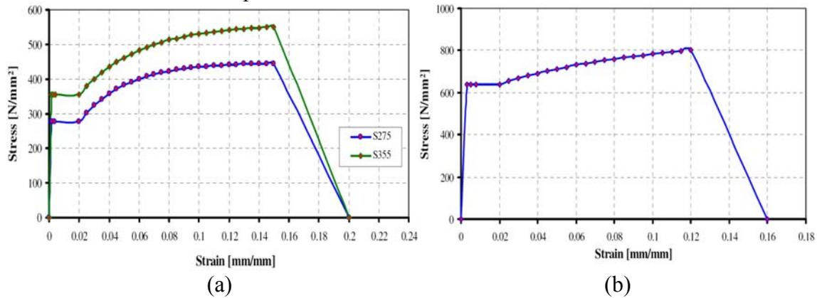
Fig. 3 - Stress-strain curves for (a) S275 and S355 steel and (b) grade 8.8 high strength bolts <sup>2</sup>
