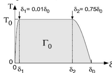
Fig. 4 - Traction-separation law for fracture <sup>12</sup>
