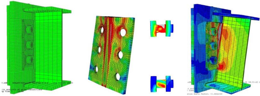
Fig. 6 - FE model of flexible end plate connection: deformed and un-deformed shapes
