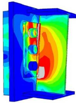
(h) Deformed shape at 550 °C
