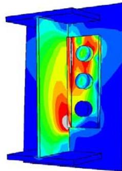
(l) Deformed shape at 650 °C
