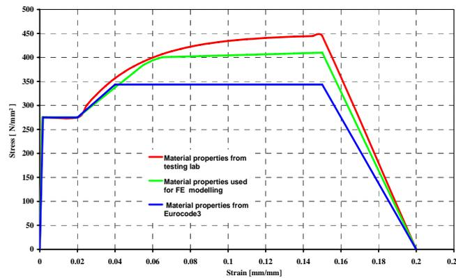
Fig. 2 - Material properties for steel
