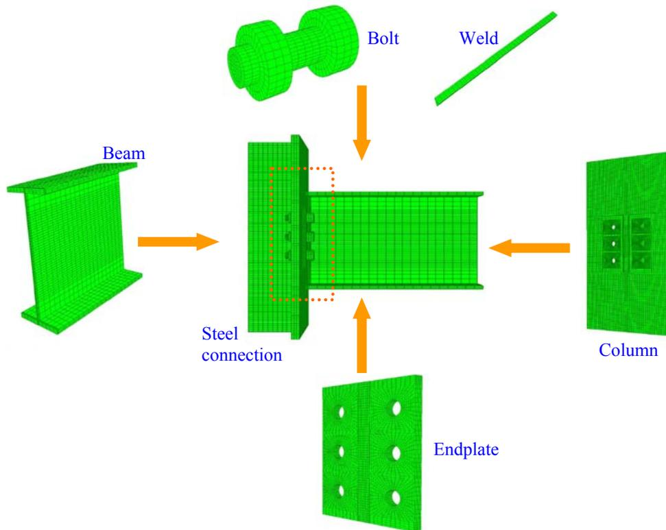
Fig. 1 - FE model for a flexible end plate connection
