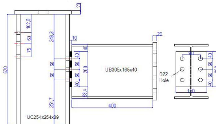
Fig. 5 - Geometrical details of the flexible endplate connection
