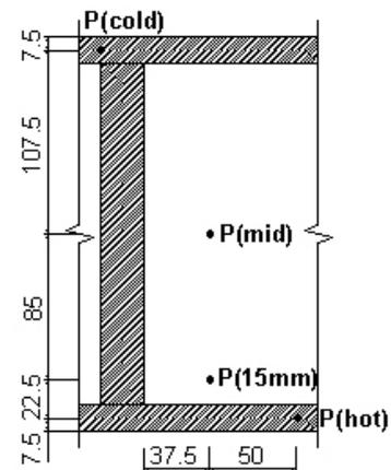
Fig. 2 – Key points used in heat transfer analysis
