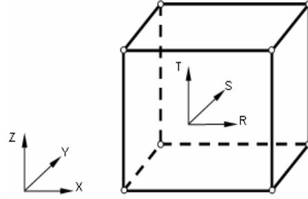
Fig. 16 – 3D eight-noded brick element
