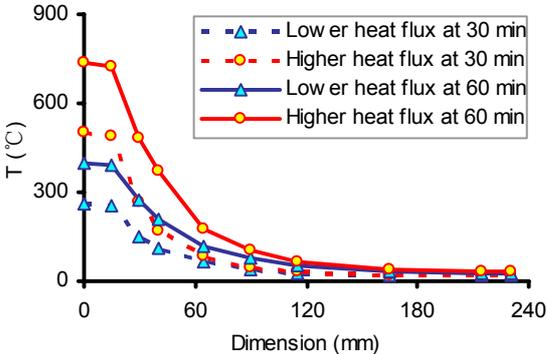
Fig. 7 – Temperature distributions along steel bar connector
