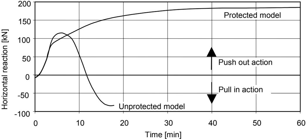
Fig. 7. Horizontal reaction at the beam-column connection under estimated loading in the standard fire.
