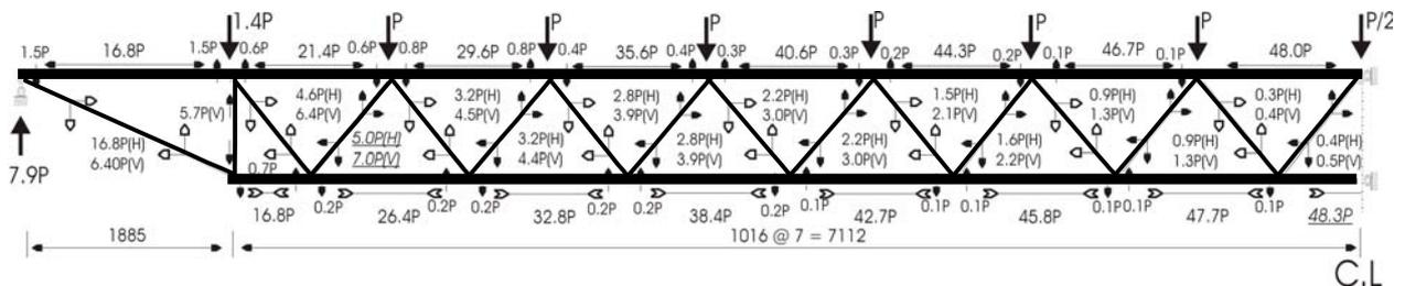
Fig. 4 Equilibrium of the unrestrained composite truss at ambient temperature
