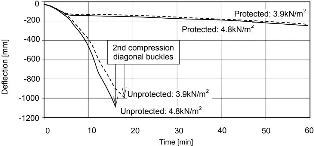
Fig. 6 Vertical deflection at the mid-span of the top chord in the standard fire.
