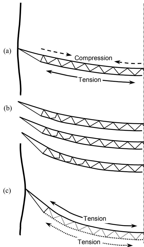
Fig 8. Equilibrium of the composite truss: (a) in bending; (b) as diagonals buckle; (c) in full catenary action.
