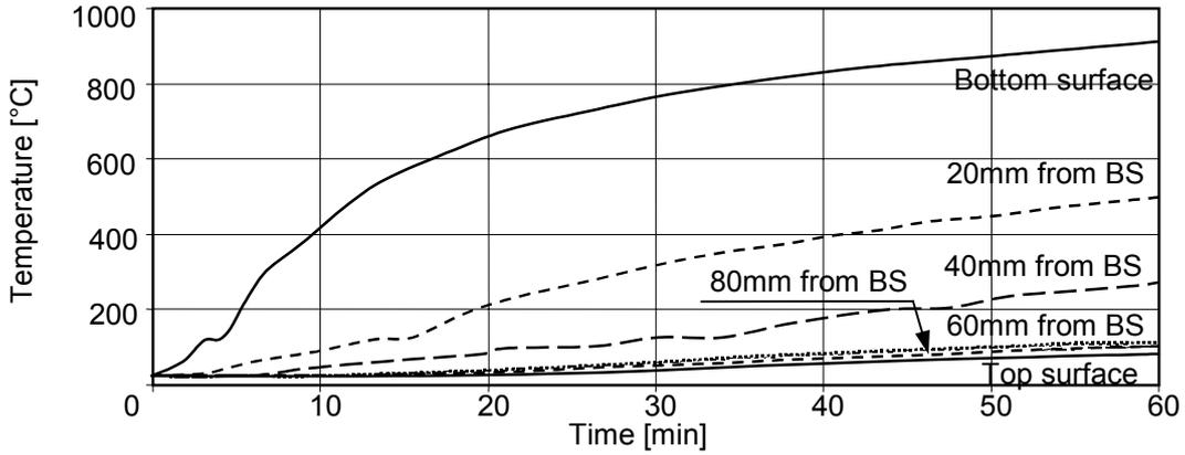
Fig. 3 Temperature development of the 100mm topping of LWC slab in the standard fire
