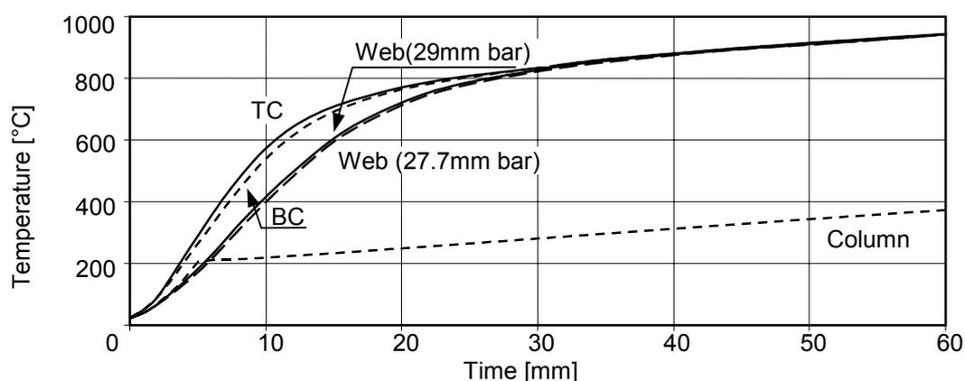
Fig. 2 Temperature development of unprotected chord members in the standard fire
