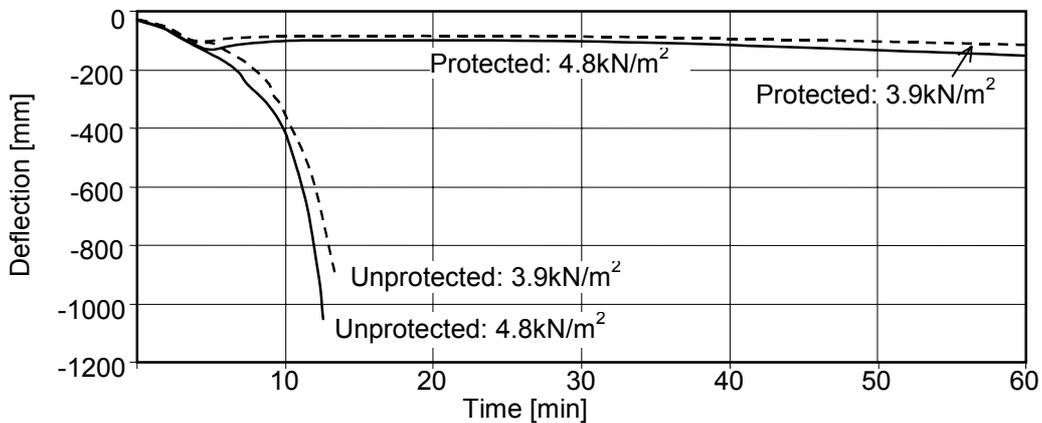
Fig 5. Vertical deflection at top chord mid-span of the simply supported truss in the standard fire
