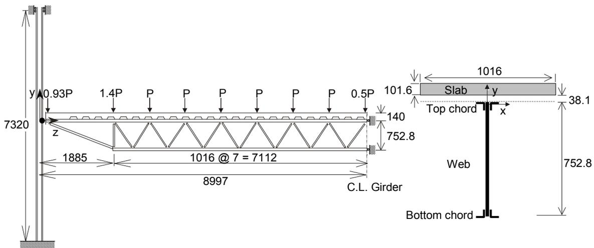
Fig. 1 Layout of the composite truss model (dimensions in mm)
