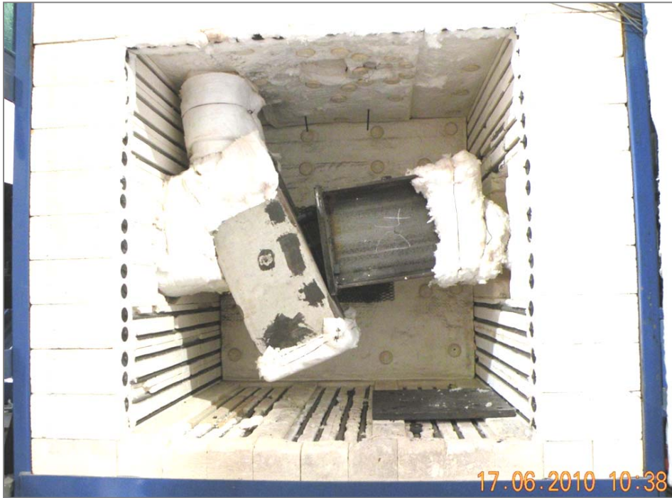
Failure mode: nut stripping of all bolts
