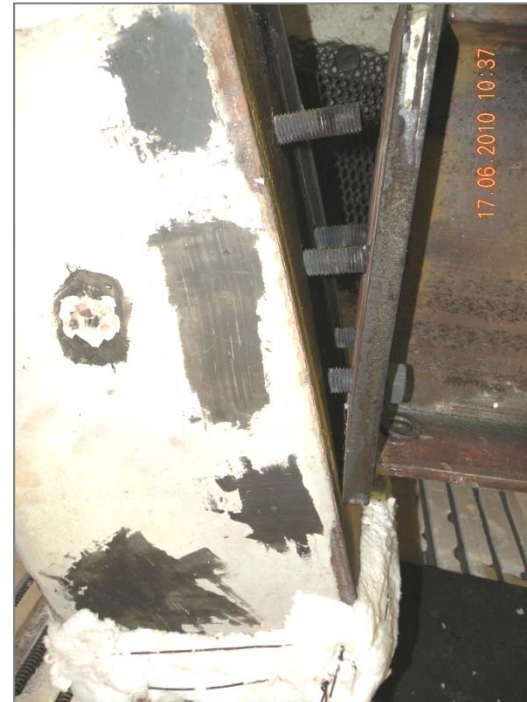
Failure mode: nut stripping of all bolts
