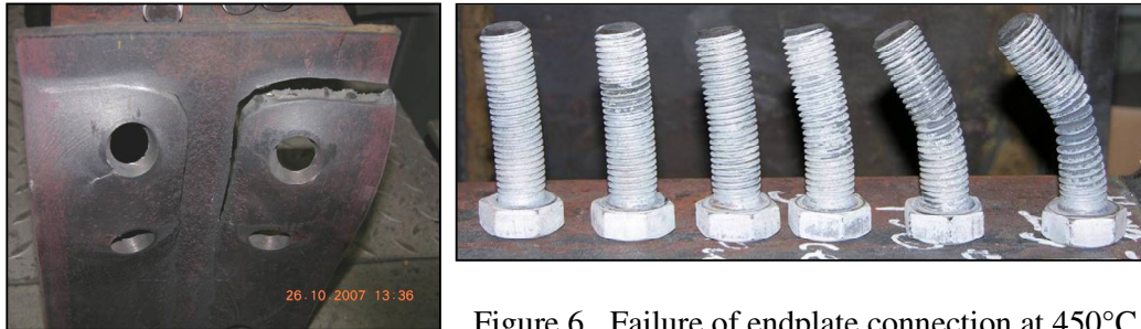
Figure 6 Failure of endplate connection at 450°C.
