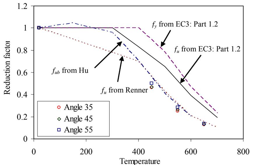
Figure 7 Reduction of the connection resistances with temperature
