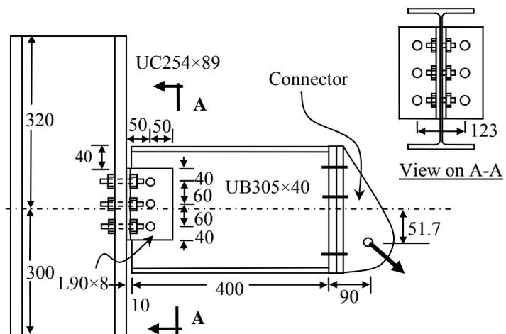
Fig. 2. Details of the test specimen
