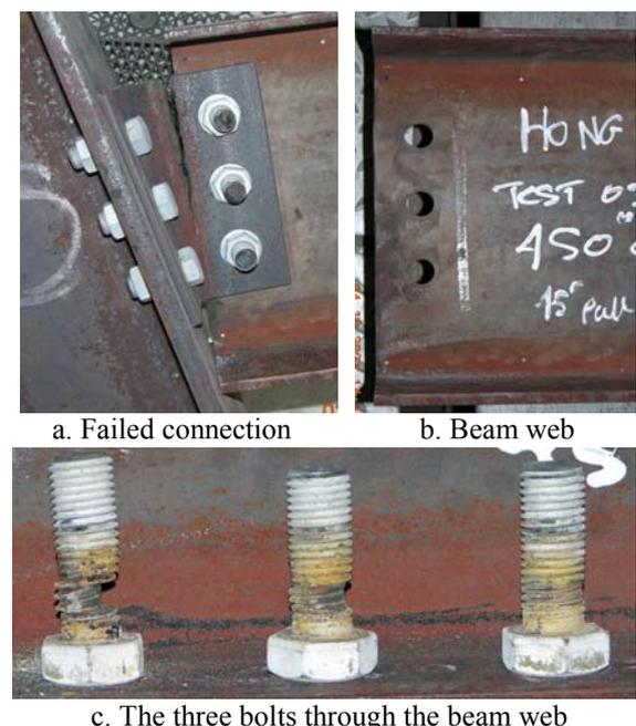
Figure 4 Failure mode at 450°C and 550°C
