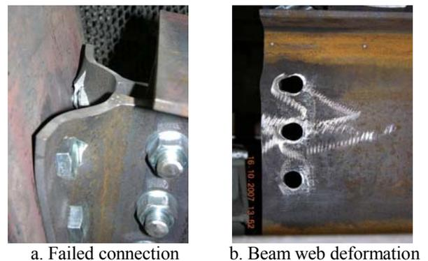
Figure 3 Failure mode at ambient temperature
