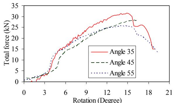
Figure 6 The force-rotation relationships of the tested connections
