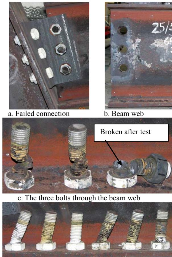
Figure 5 Failure mode at 650°C
