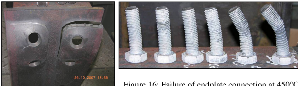
Figure 16: Failure of endplate connection at 450°C.
