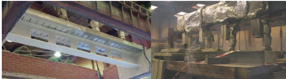
Figure 3. Experimental setup: Beam within the furnace, apply loads on beam.
