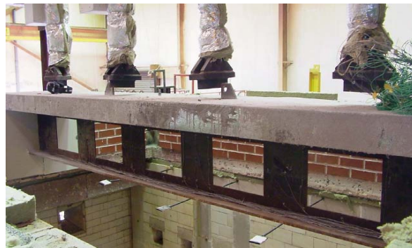
Figure 2: Experimental setup: loads applied to beam
